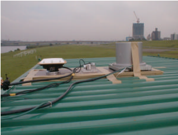
Figure 1. Setup of the UNSW-MRI GPS Seismometer Experiment.
