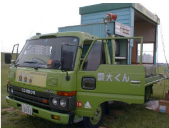
Figure 2. Earthquake shake-simulator truck used in the UNSW-MRI GPS Seismometer Experiment.
