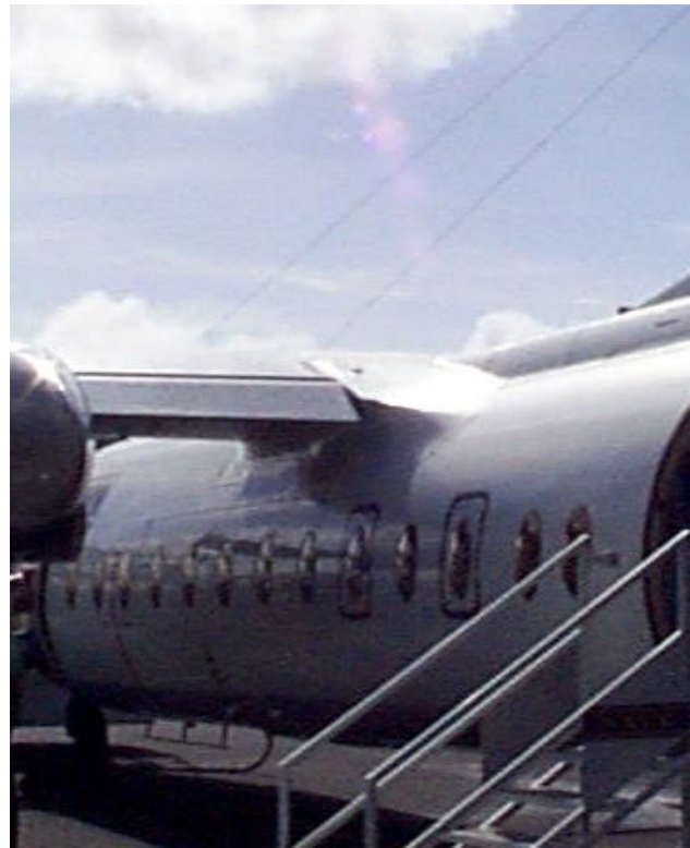
Fig. 3. The small "bumps" in the middle of both photos, on the upper surface of both wings, are GPS antennas (NovAtel 512). The horizon from the antenna is 12 degrees up to the fuselage top and 10 degrees up to the wing top. The antenna on the left figure was used for the Torres Strait experiment, and both antennas were used for the Lake Argyle experiment.
