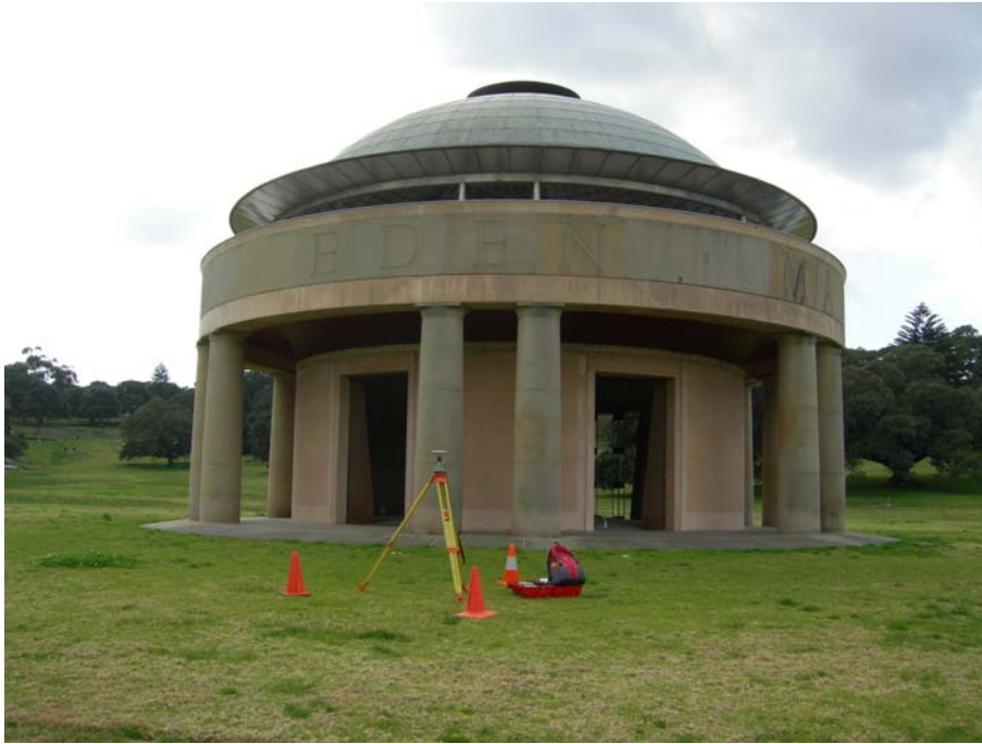
Figure 3: Rover receiver in Centennial Park, Sydney.
