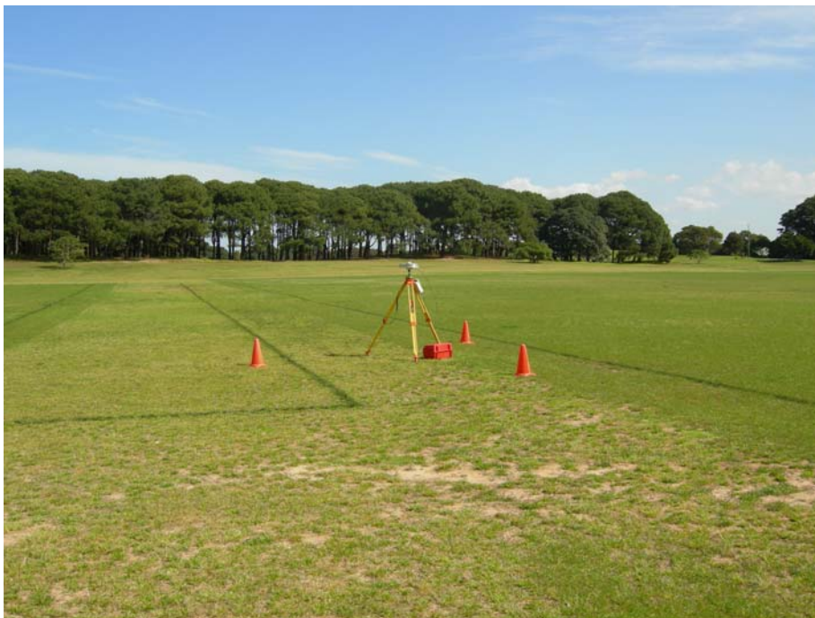
Figure 4: Base receiver in Centennial Park, Sydney.
