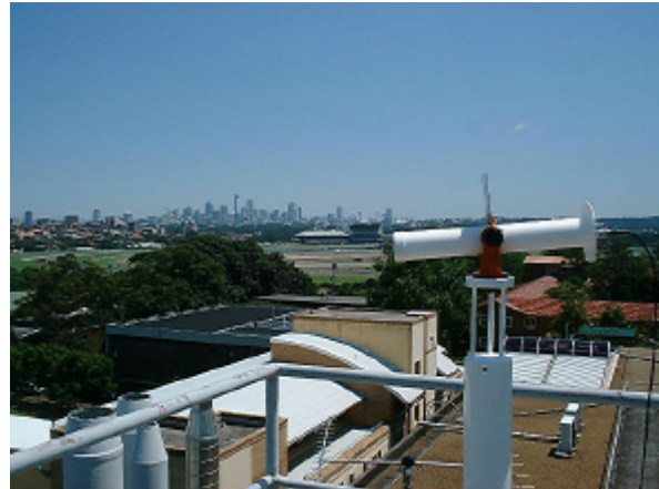
Figure 6: Helical antenna of the reference pseudolite (PL32).
