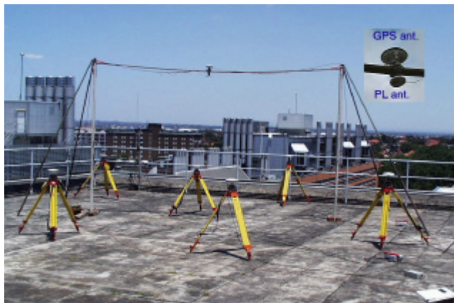
Figure 4. Test configuration of the GPS/PL system at UNSW.
